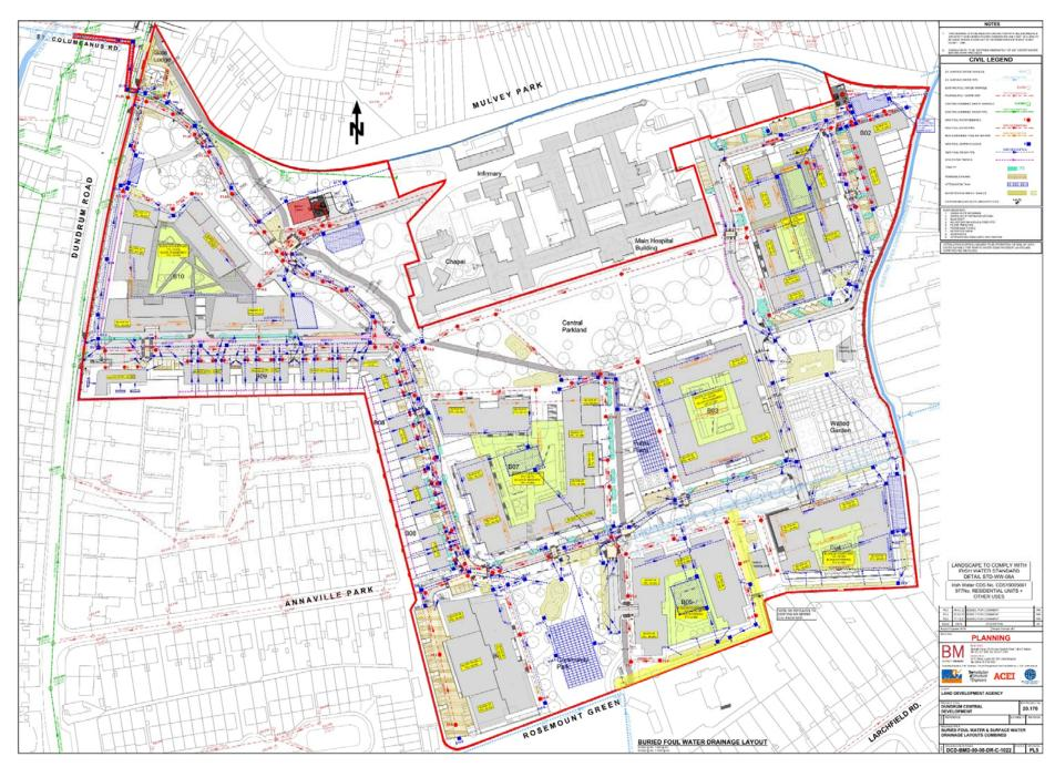
Figure 8. Buried foul and surface water drainage network
